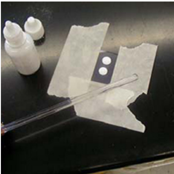
Image 03: forming a tape mold w/sample on a slide
