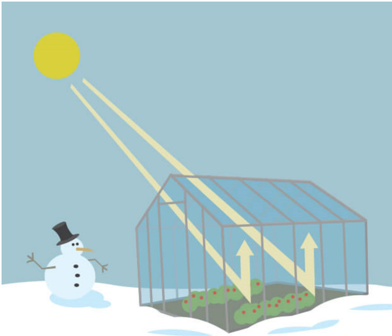
Figure 4: A greenhouse captures heat from the Sun during the day. Its glass walls trap the Sun's heat, which keeps plants inside the greenhouse warm - even on cold nights. Credit: NASA/JPL-Caltech
