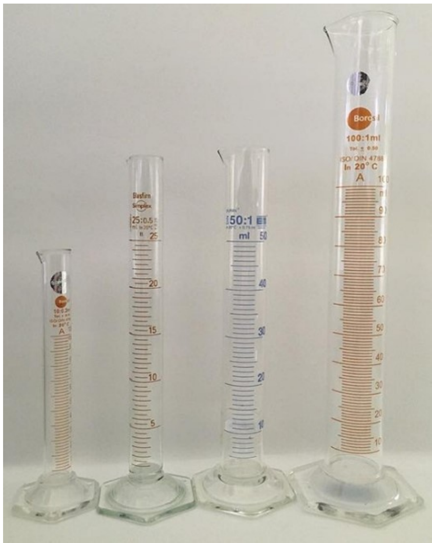
Figure 3: Graduated Cylinders. Four glass graduated cylinders of various sizes that measure from left to right 10, 25, 50 and 100 milliliters (mL). 33
